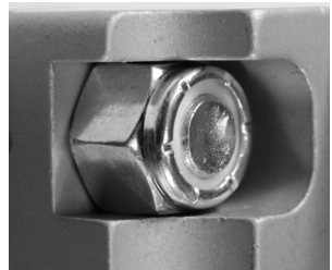
fig. 21: Bolt protrudes just beyond flush
