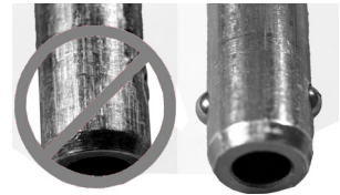
fig. 31: Left pin – retired due to wear and detent pins not properly working; Right pin – in good working condition
