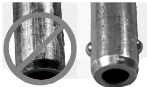
fig. 18: Left pin – retired due to wear and detent pins not properly working; Right pin – in good working condition
