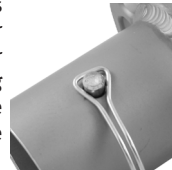
fig. 2: Properly secured Leg Coupling Pin
